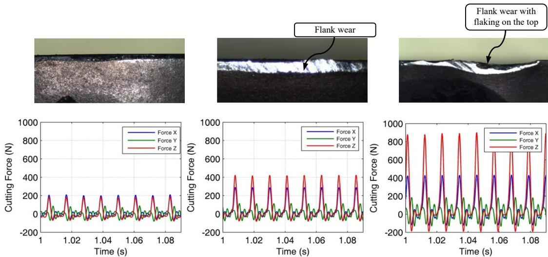
Figure 2. The cutting forces during milling process: (a) at flank wear = 0.144 mm, (b) at flank wear = 0.242 mm, and (c) at end of cutting, flank wear = 0.519 mm.
