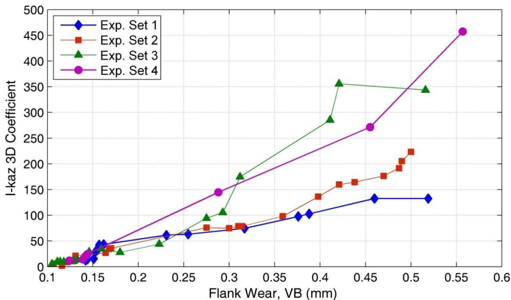
Figure 4. I-kaz 3D coefficient against flank wear.
