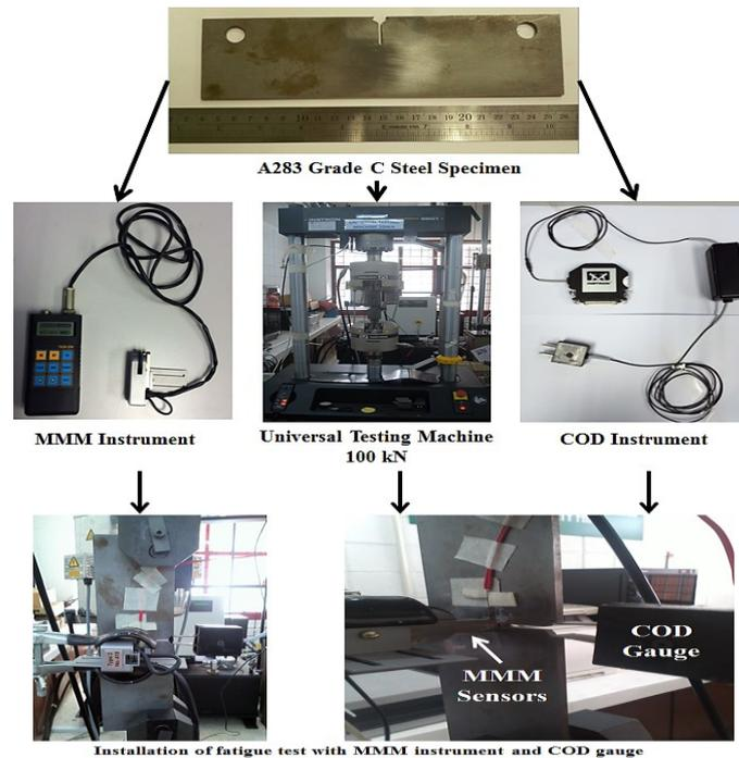
Figure 1. Overall process flow of the experimental procedure.
