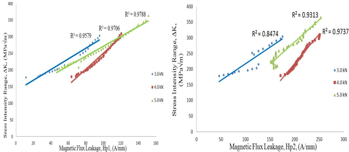
Figure 6. Correlation of stress intensity range,  $\Delta K$  and magnetic flux leakage,  $Hp(y)$ .
