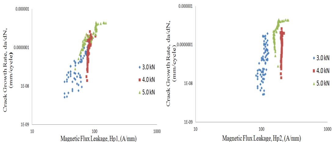
Figure 5. Crack growth rate curve ( $da/dN$  versus  $H_p(y)$ ).
