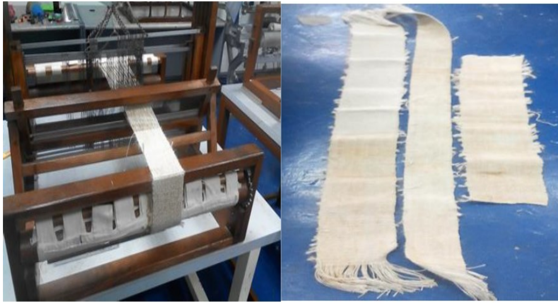
(a) (b) Figure 2. (a) In-house weaving machine and (b) Finished woven type fiber mats.
