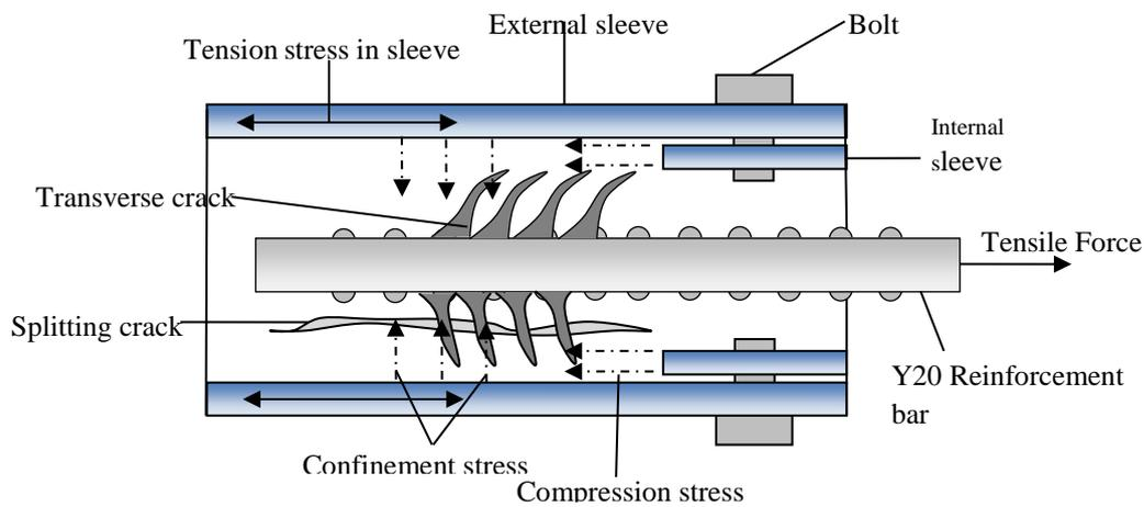
Figure 6. Load transfer mechanism in grouted sleeve connector.
