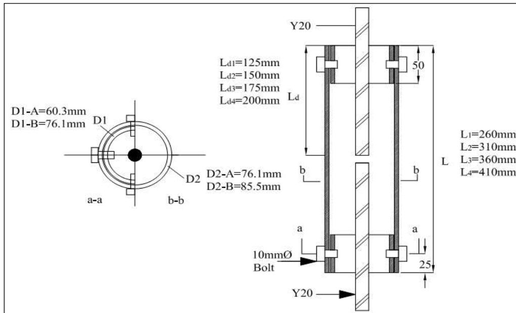
Figure 1. Detailing of grouted splice sleeve connector.
