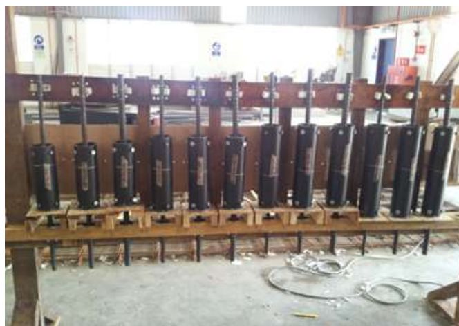
Figure 2. Grouted splice sleeve connector tied to wooden frame.
