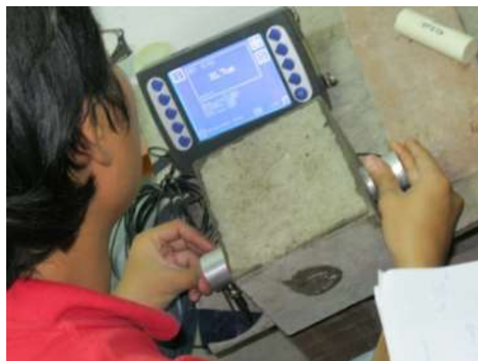
Figure 4. UPV measurement of concrete specimen.
