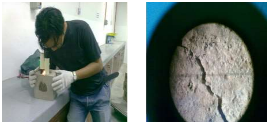
Figure 3. Pre-cracked hairline measurement on concrete specimen under microscope.
