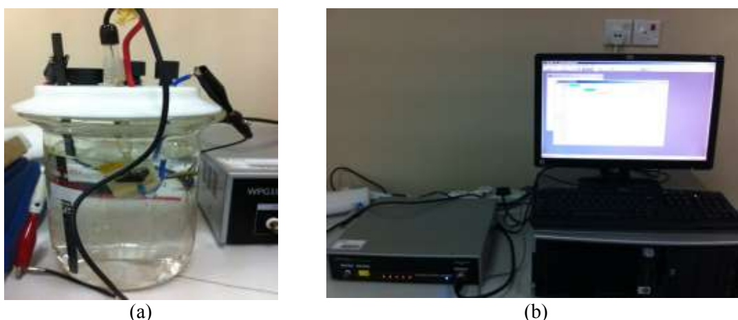
Figure 2. Potentiodynamic polarization set-up: (a) electrochemical measurement set-up; (b) WPG100 potentiostat.
