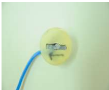
Figure 3. Working electrode consisting of weld metal and base metal.
