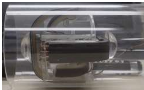
Figure 2. Photograph of the magnetic actuator system.
