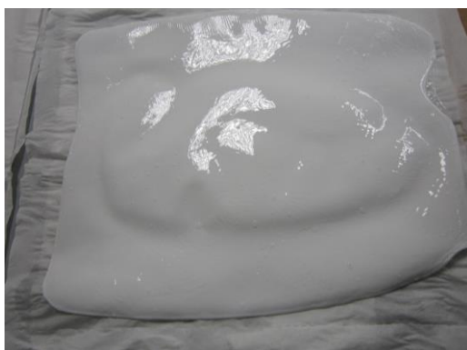
Figure 2. Polyethersulfone membrane after immersion in distilled water.
