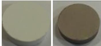
Figure 1. Green and fired sample with electrode.
