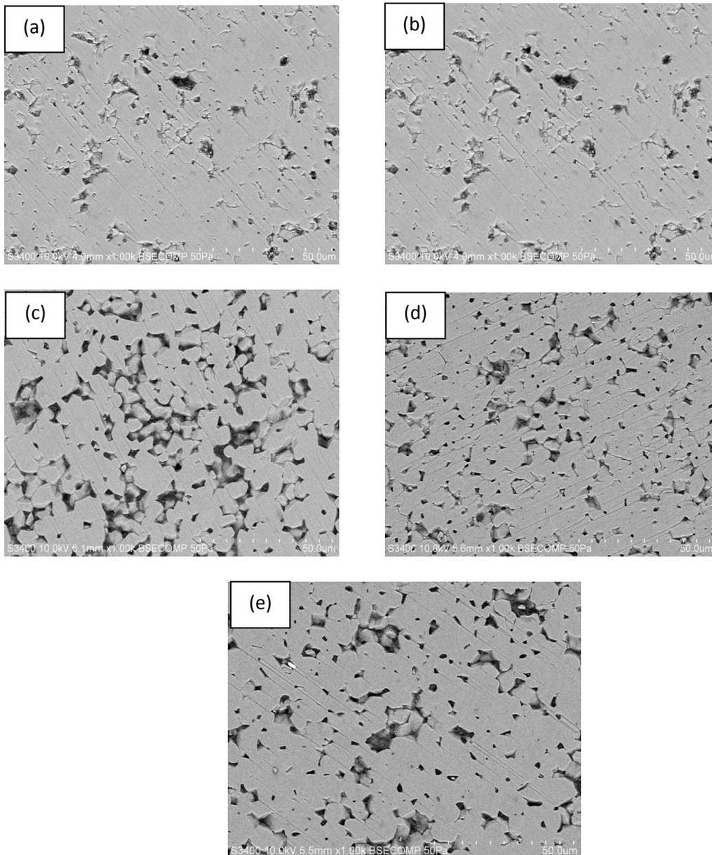
Figure 3. SEM photomicrographs with different concentrations of  $WO_3$ : (a) 0.2%  $WO_3$ , (b) 0.4%  $WO_3$ , (c) 0.6%  $WO_3$ , (d) 0.8%  $WO_3$ , (e) 1.0%  $WO_3$
