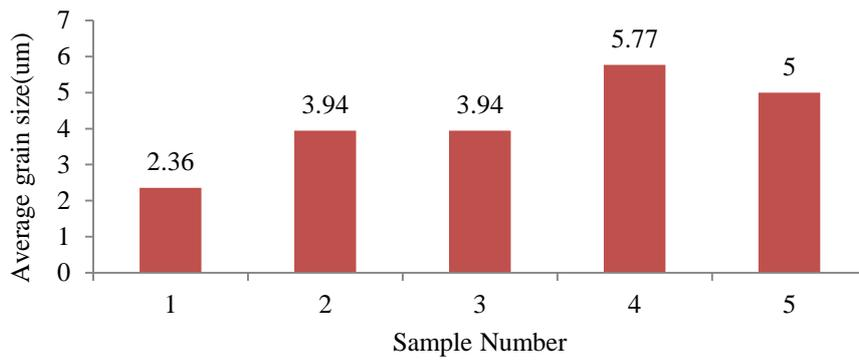
Figure 2. Average grain size with different concentrations of  $WO_3$ .
