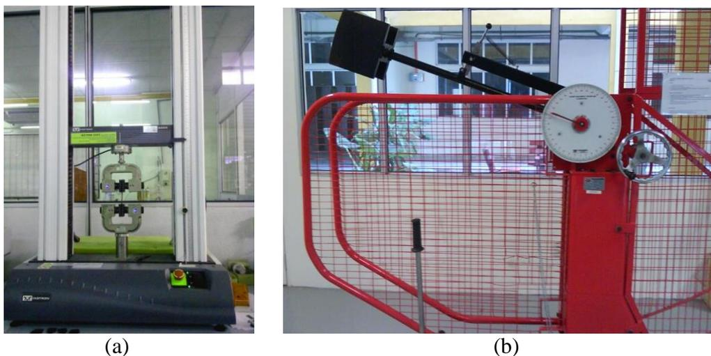
Figure 2. (a) Universal Tensile Machine (UTM); (b) Izod impact testing machine.
