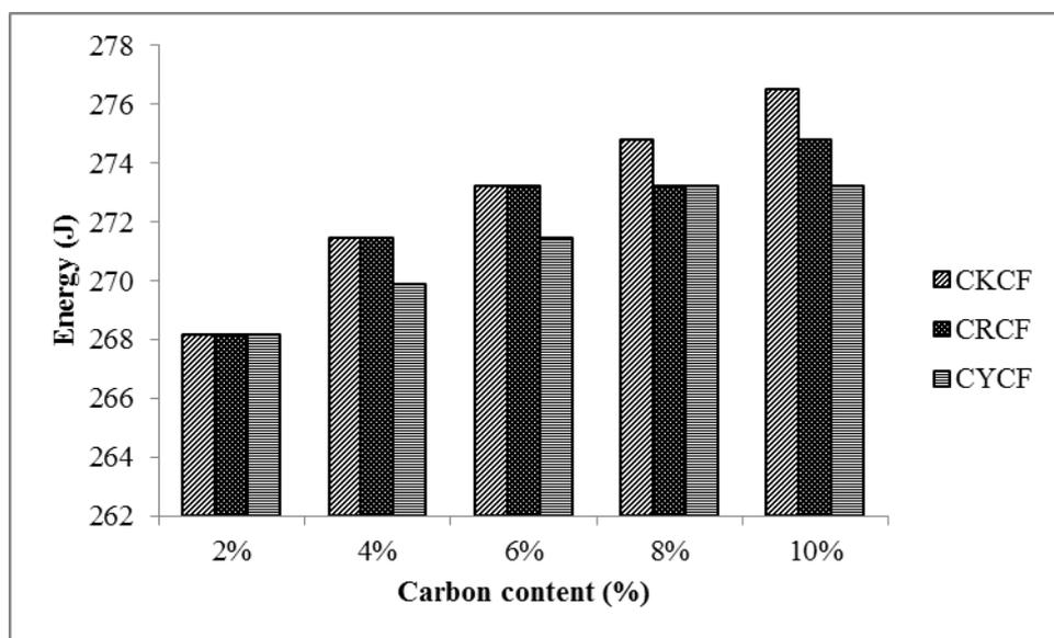
Figure 4. Izod impact strength for CKCF, CYCF and CRCF composites.
