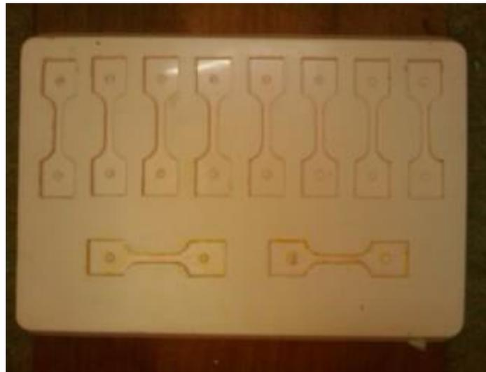
Figure 1. Silicon rubber mold (SRM)
