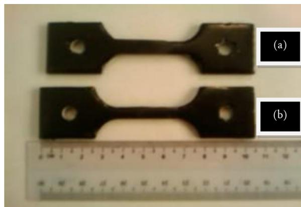
Figure 6. Differences in length of specimens after creep testing.
