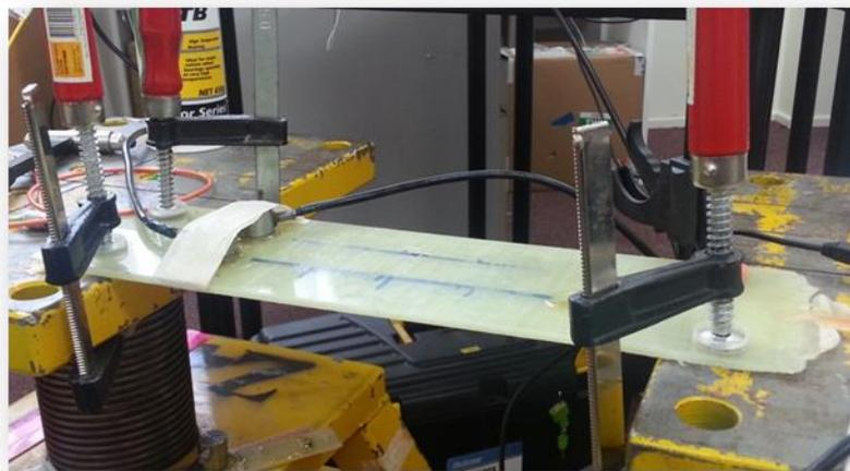
Figure 4. Specimen prepared before the low frequency impact by hammer.
