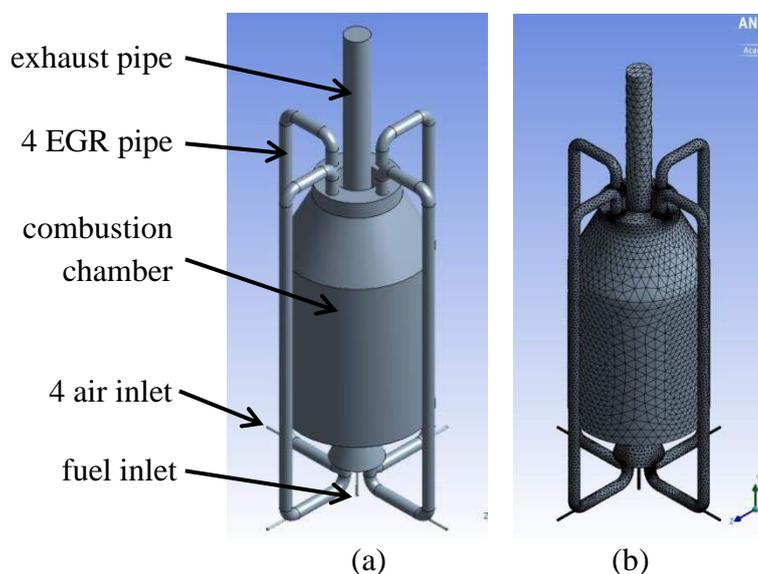
Figure 2. Final design with bigger EGR pipe: (a) schematic diagram with boundary condition; (b) model after meshing
