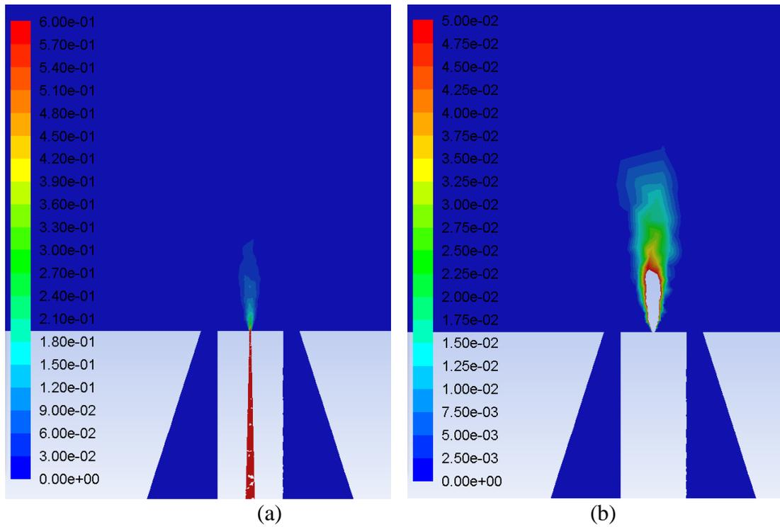
Figure 5. Mole fraction of CH<sub>4</sub> species (a) between 0 and 0.6 (b) between 0 and 0.05
