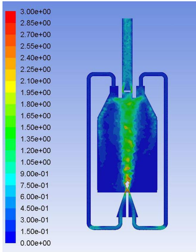
Figure 3. Velocity magnitude inside the combustion chamber
