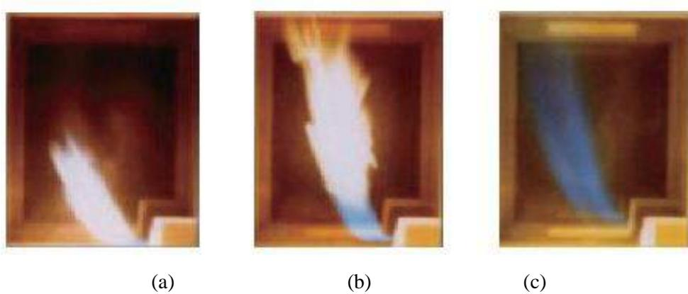
Figure 1. Combustion air temperature of 1100°C and percentage of O<sub>2</sub> concentration: (a) 21% oxygen, (b) 8% oxygen, (c) 2% oxygen (Gupta et al., 1999)
