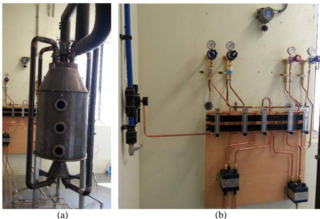
Figure 8. MILD burner setup: (a) with three glass windows; (b) gas control panel
