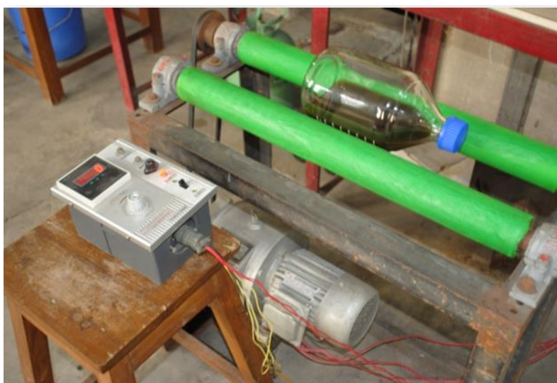
Figure 3. Locally fabricated ball mill
