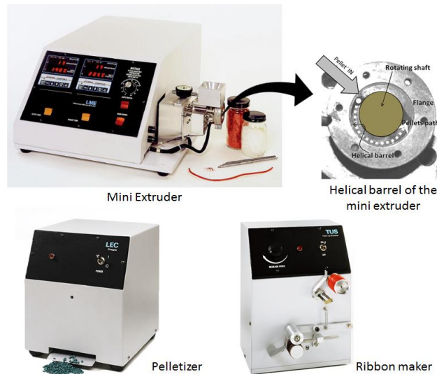
Figure 2. Laboratory Mixing Extruder complete with its pelletizer and ribbon maker.
