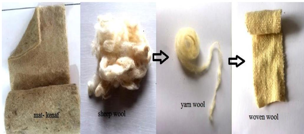
Figure 1. Materials used in this study. (a) kenaf mat (b) sheep wool, yarn and wool woven
