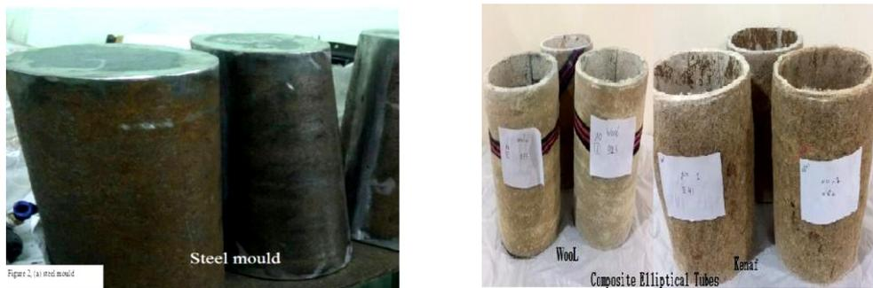
Figure 2. Steel mould and both test samples are ready for crushing test (WRCEC), (KRCEC).
