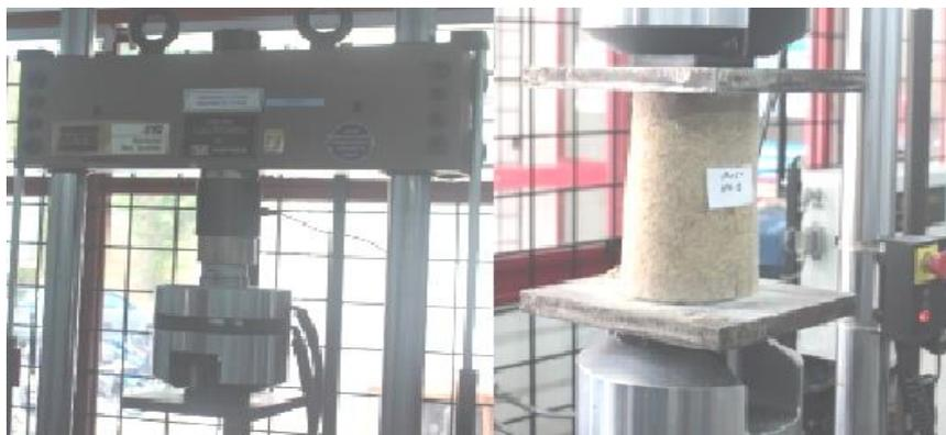
Figure 3. Instron machine types MTS 810 (25 Tones) and test fixture.
