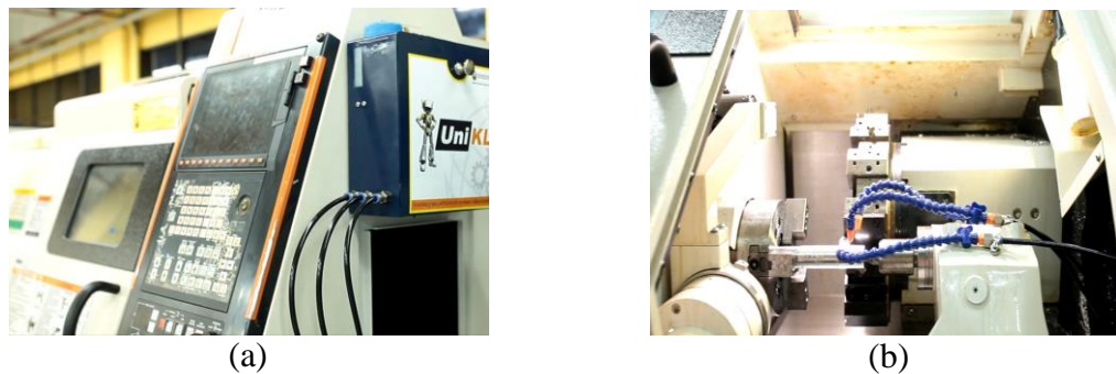
Figure 3. (a) Portable MQL applicator was installed on the CNC lathe machine (b) nozzle orientation.
