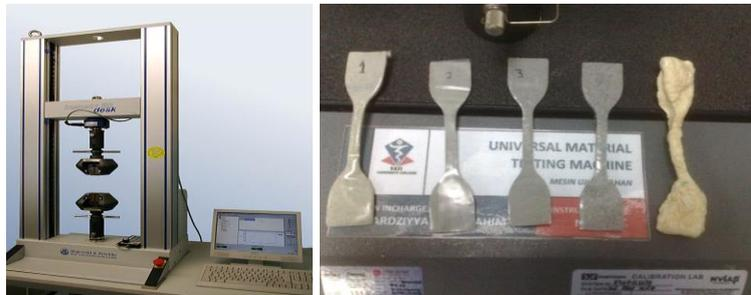
Figure 3. Instron Universal Testing Machine for tensile testing and the dumbbell shaped samples.
