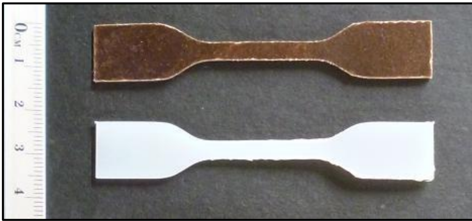
Figure 2. Tensile specimens of neat HDPE (below) and K-HDPE composite (above).
