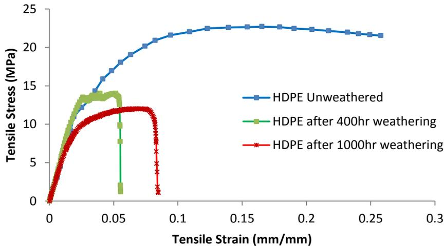
Figure 8. Stress-strain curves of weathered and unweathered HDPE.
