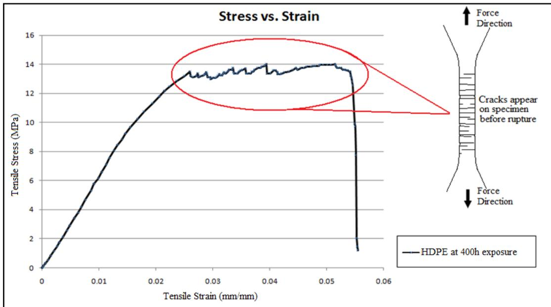
Figure 5. The stress-strain curve of the weathered HDPE at 400 h of exposure.
