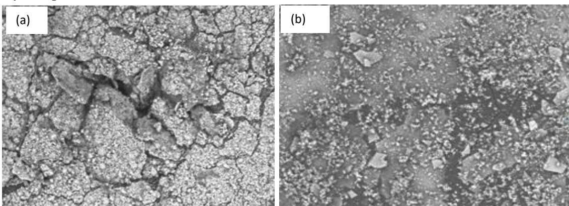
Figure 5. (a) Paint 1 and (b) Paint 3 after 60 days of immersion in seawater.
