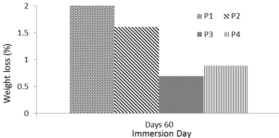
Figure 3. Bar chart of the weight losses for Paint 1, Paint 2, Paint 3 and Paint 4 for 60 days immersion.
