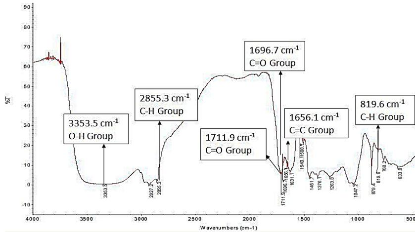
Figure 2. IR spectra for henna extraction by using FTIR analysis.
