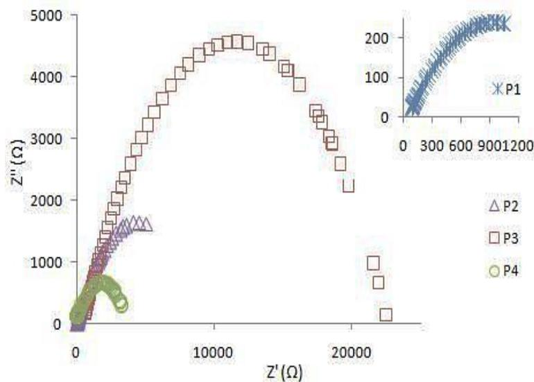
Figure 4. Nyquist plot of specimen immersed in seawater for 60 days.
