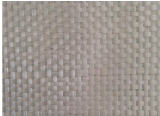
Figure 1. Woven Roving glass fibre single ply.
