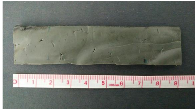
Figure 1. Example of SMR CV-60 specimen for tensile test.
