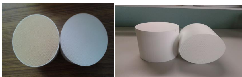
Figure 2. Ceramic honeycomb monolith substrate.
