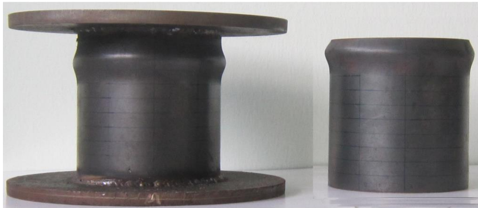
Figure 3. The collapse cylinders bulging out in the neighborhood of one end of the cylinder.
