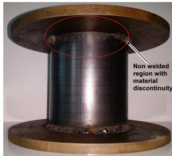
Figure 5. Cylinder CY5 with introduced circumferential material discontinuity on the top flange.
