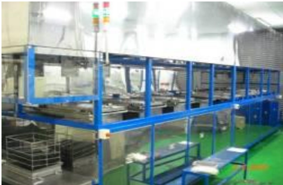
Figure 2. Automatic hydrocarbon washing machine and experimental setup
