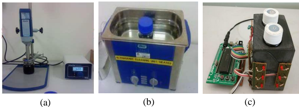
Figure 1. Steps used in the preparation of nanofluids (a) homogenisation process; (b) sonication process; (c) stability process.
