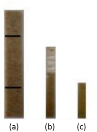
Figure 2. Sample of natural fiber composites according to ASTM Standards; (a) Tensile test (ASTM D3039), (b) Flexural test (ASTM D790), (c) Impact test (ASTM D256).
