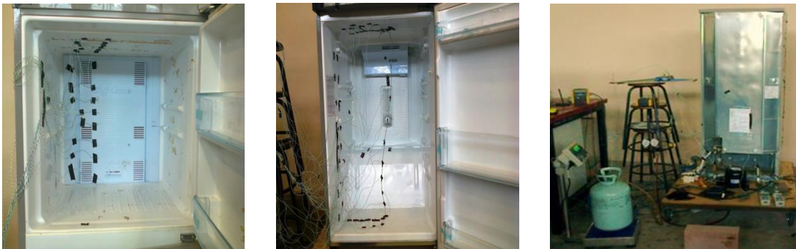
Figure 4. Experimental rig: (a) freezer thermocouples, (b) refrigerator thermocouples, (c) instrumentation.
