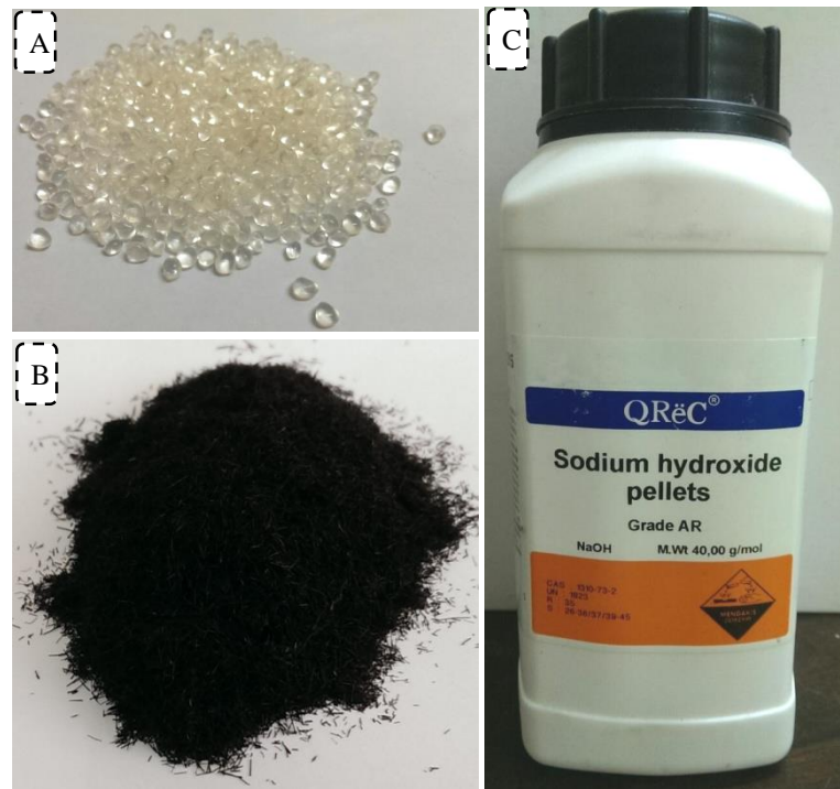
Figure 1. (a) Pure TPU, (b) SPF, and (c) sodium hydroxide.
