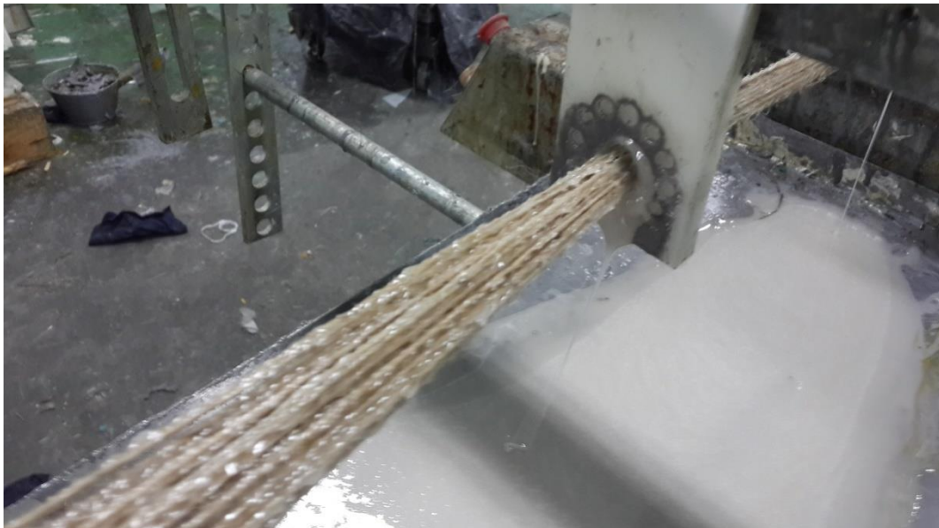
Figure 1. Production of kenaf reinforced vinyl ester composite rod: resin-impregnated fibres were pulled through a guide plate before entering a heated die (courtesy of Innovative Pultrusion Sdn. Bhd., Seremban, Malaysia).
